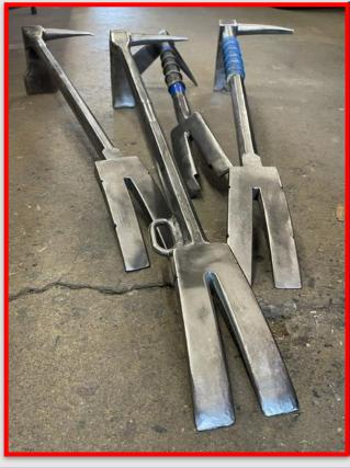
THE MOST VERSATILE TOOL USED IN THE AMERICAN FIRE SERVICE IS THE HALLIGAN BAR. THIS SIMPLE TOOL HAS SO MANY USES AND CHARACTERISTICS THAT ARE OFTEN OVERLOOKED. DURING THIS ONE DAY CLASS, WE ARE GOING TO BREAK DOWN THE HALLIGAN PIECE BY PIECE.
